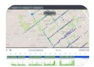
GPS device on the machine helps to identify speed graphics in case of over-speeding or vehicle standing idle. In case of deviations from the assigned route, SMS alerts are sent to official mobile numbers for immediate rectification.
